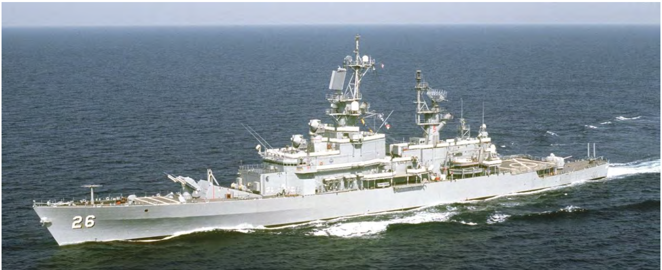
USS Belknap (CG 26) after being reconfigured for Flagship Duty. Notice the new “box” on the main deck below the pilot house. Among other changes, the helicopter hanger was also removed.
